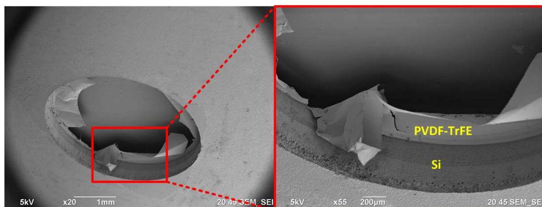
Figure 4.7: SEM image of an actuator-membrane device.
